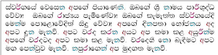
Fig. 11.9. The illustration of a segmentation-free OCR for Sinhala text (Sri Lanka), implemented by use GST, after [186]. The points are painted colored at the places where a support for a GST character template has been found
