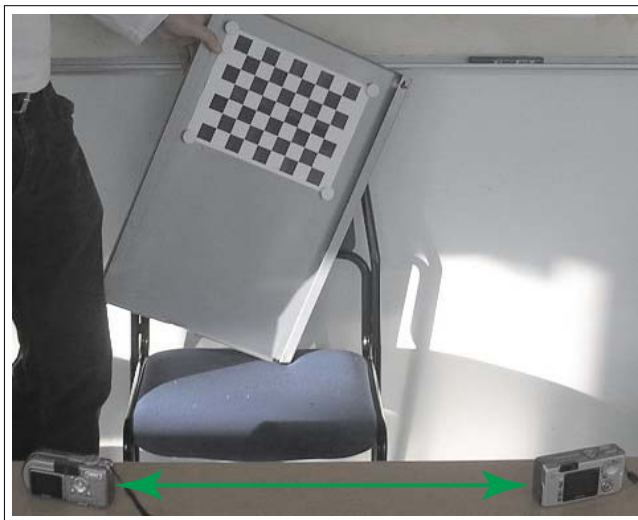
Fig. 13.4. The checkerboard consists of black and white squares with side lengths of 28 mm. Such patterns are frequently used to calibrate cameras, i.e., their intrinsic and extrinsic parameters are computed
