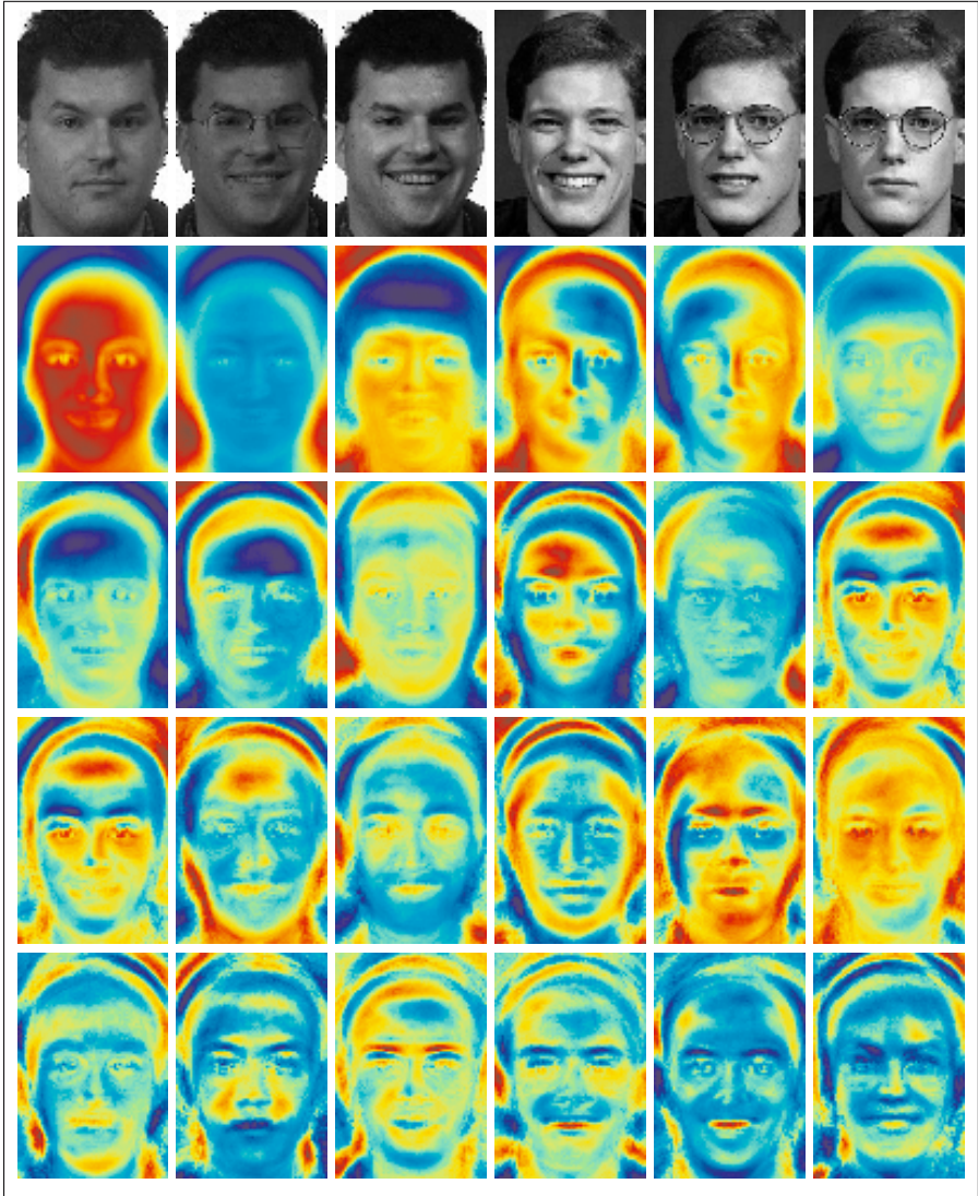
Fig. 15.1. Top row shows samples of 64 \times 96 face images of two persons [154]. The color images show the 24 most significant basis faces that are found by PCA
